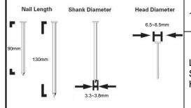
15° flat wire welded coil nails
