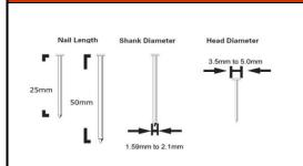
15° conical wire welded nails and flat plastic sheet collated nails
